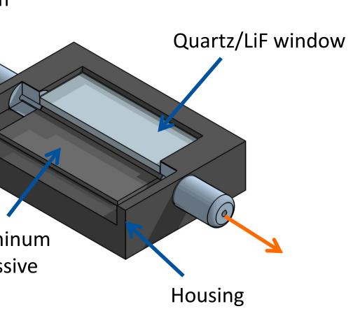
Ionization takes place in an ion source integrated into an inlet capillary. A UV- or VUV-lamp mounted on top of the ion source provides the light for photoelectron generation (APECI) or for single photon generation (APPI). A flute milled inside the metal leads to an identical gas flow as compared to standard capillaries. The photoemissive material is anodized aluminum.
