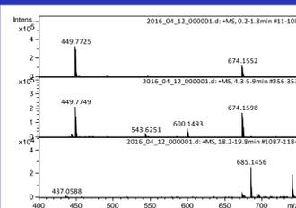
**Figure 2a:** Mass spectra of Substance P at different in source CID potentials, 15 V (top), 50 V (center) and 300 V (bottom); minute activation leads to fragmentation of the triply protonated molecule (m/z 499.8), strong activation results in complete loss of [M+3H]<sup>3+</sup> and poor overall ion transmission
