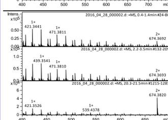
**Figure 2c:** Mass spectra of Substance P at different CID potentials, 15 V (top), 65 V (center) and 300 V (bottom), with 3.3 % methanol added to the background gas; increasing the CID potential results in decrease of the MeOH-H<sub>2</sub>O cluster abundance,
