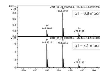
**Figure 3b:** Mass spectra of Substance P obtained at different background pressures in the inlet stage, background gas saturated with acetonitrile
