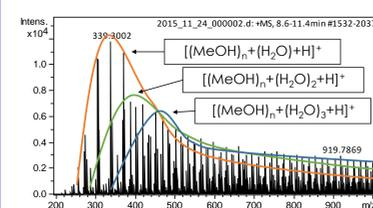
**Figure 1c:** Mass spectrum showing series of solvent clusters; 4.9% methanol added to the background gas; at higher MeOH mixing ratios the distribution is shifted to higher numbers of MeOH clusters
