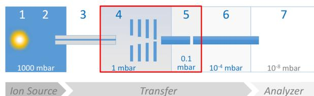
In a thermodynamically controlled elevated pressure region the formation of bare gas phase ions is unlikely, as protonated molecules will readily interact with polar substances present in the background gas for charge stabilization (formation of e.g. protonated analyte-solvent clusters or protonated dimers). Ion activation will ultimately lead to cluster dissociation, transferring the proton to the compound with higher proton affinity.
