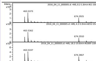
**Figure 2b:** Mass spectra of Substance P at different CID potentials, 15 V (top), 50 V (center) and 300 V (bottom), with 5.9 % acetonitrile added to the background gas leads to formation of analyte-acetonitrile clusters. Increasing the CID potential results in higher signal intensities, no fragmentation is observed
