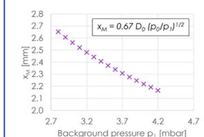
**Figure 3a:** Calculated distance  $x_M$  between the inlet capillary exit and the Mach disc as a function of the background pressure in the first vacuum stage
