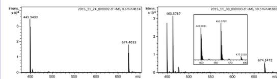
**Figure 1a:** nanoESI mass spectrum of Substance P diluted in 50% aqueous acetonitrile with 0.1% formic acid (left); background gas in the ion source saturated with acetonitrile leads to M+nACN cluster formation, but only for the triply protonated molecule (right)
