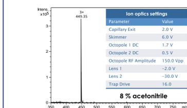
**Figure 1e:** No MeCN clusters were detected with the ion trap instrument, even at very mild transfer and trapping settings
