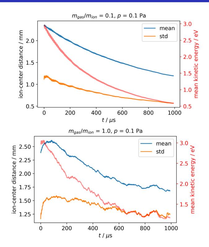
**Right:** Kinetic energy evolution over time of single ions, the red lines indicate collisions.
