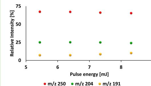
Figure 4: Fragmentation behaviour in dependence of the laser intensity of the focused Nd:YAG laser system
