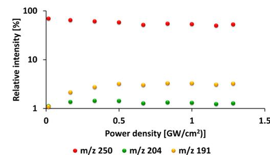
Figure 3: Fragmentation behaviour in dependence of the laser energy of the focused excimer laser system. Note log intensity scale.
