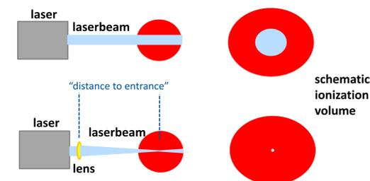
Figure 1: Schematic pathway of the laser beam and resulting ionization volume with and without focusing of the beam.
