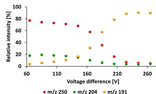
Figure 2: Fragmentation behaviour (CID) in dependence of the potential between transfer capillary exit and skimmer
