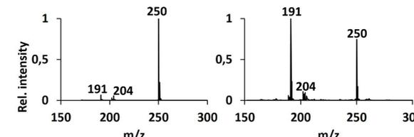
Figure 7: Fragment spectrum of APA obtained with unfocused (left) and focused (right) excimer laser radiation
