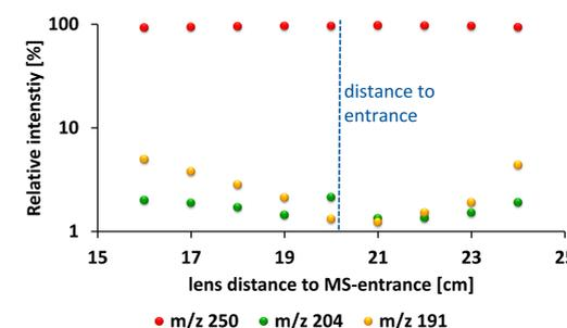
Figure 6: Fragmentation behavior in dependence of lens distance to the mass spectrometer sampling orifice
