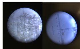
Figure 5: damaged Quartz glass window after laser irradiation (excimer/ Nd:YAG) in 10x magnification
