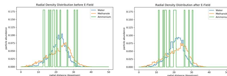
Fig. 5: Radial distribution of molecules within the droplet (left: before E-field, right: after E-field). The radial distribution is the average radial abundance of a particle species in the simulation measured from the center of mass.
