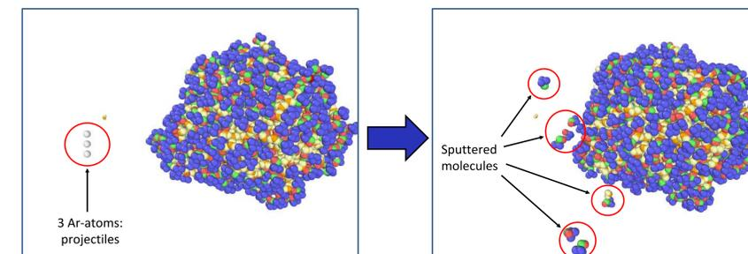
Fig. 7: Molecules are sputtered from the surface of the droplet (left: before collision, right: after collision)
