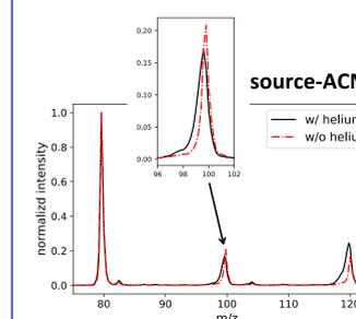
**Above:** In case of the cluster species peak fronting is observed. Decreasing the collision rate by switching off the helium buffer gas improves the peak width and symmetry. Dissociation of the fragile ions is inhibited. The shape of the stable  $MH_2^{2+}$  signal remains unchanged.
