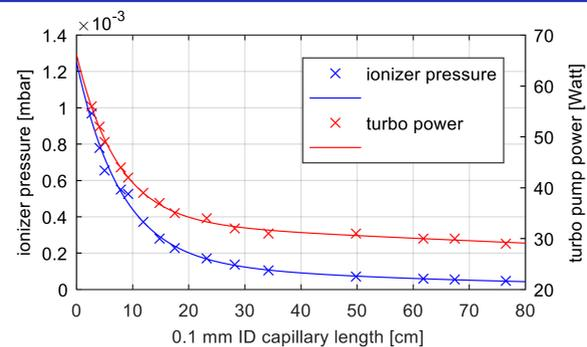
Figure 2: Ionizer pressure and turbo pump power as a function of the flow restricting capillary length (0.1 mm ID)
