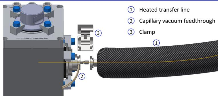
Figure 1: Schematic drawing of the transfer setup consisting of a capillary vacuum feedthrough into the EI-source (left) and a heated transfer line (right)
