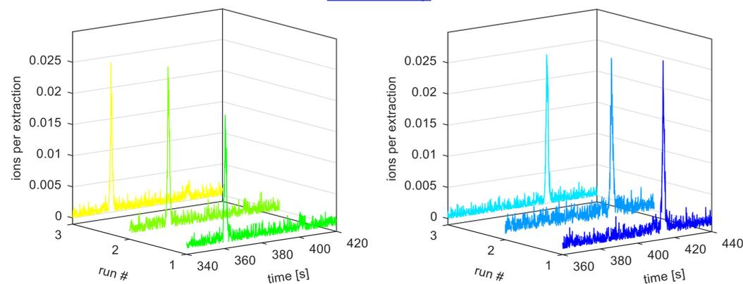
Figure 4: Chromatograms for 1 pg octafluoronaphthalene (OFN) on column. Left: conventional setup, right: flexible setup
