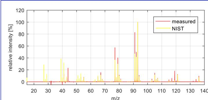
Figure 3: Background subtracted electron ionization mass spectrum of  $\alpha$ -Pinene
