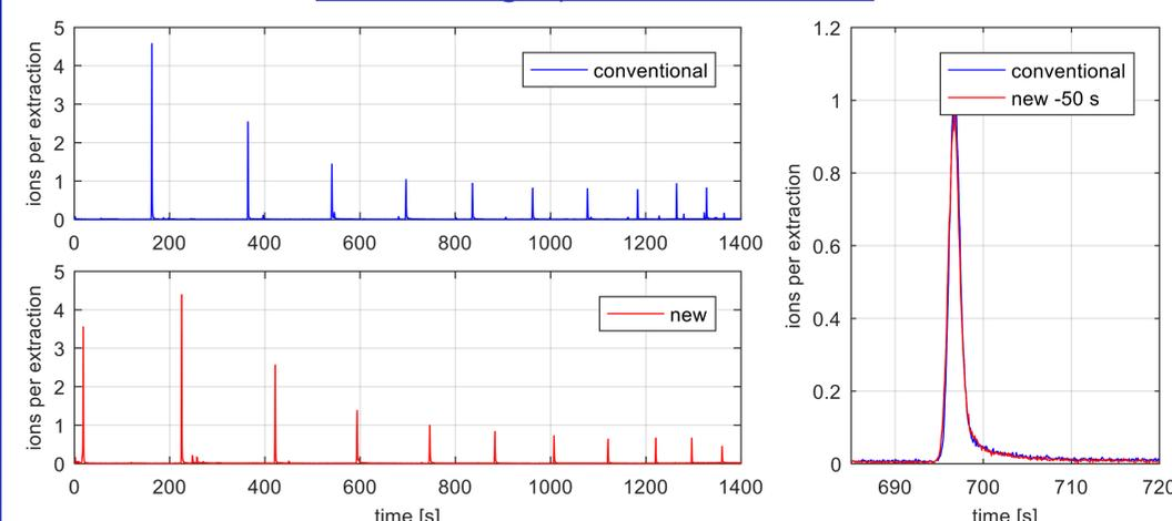
Figure 5: Comparison of chromatographic resolution between both tested setups. Left: complete FAMES chromatogram, right: signal of methyl laurate
