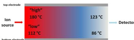
**Left:** Temperature measurements within the DMS cell at the temperature settings "low" and "high" reveal a temperature gradient.
