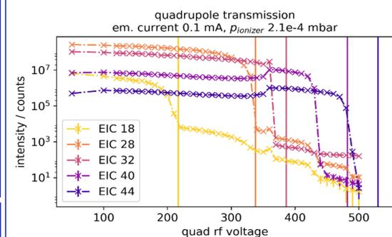
Fig. 2: At higher pressures the ions are not filtered out entirely
