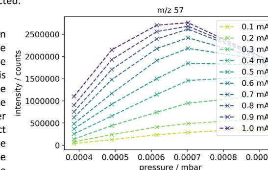
Fig. 3: Decane signals run through a maximum before declining again
