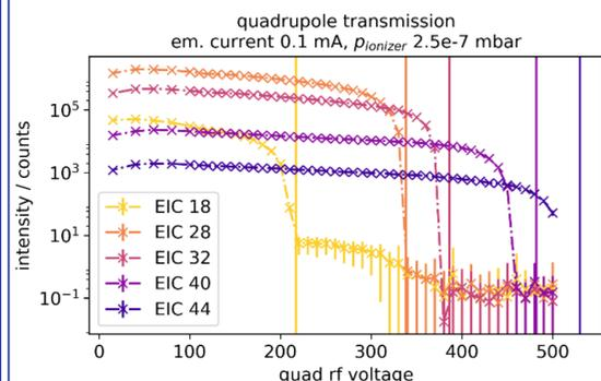
Fig. 1: Ions are successfully filtered out at their cut off voltage
