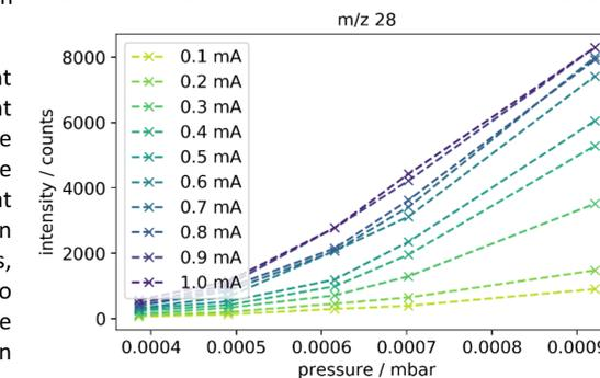
Fig. 4: Nitrogen signal increase at higher pressures even though it should be filtered out
