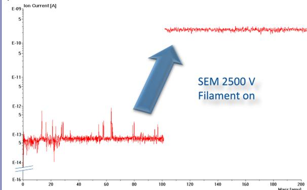
Fig. 5: The baseline goes up by 3 orders of magnitude when the filament is turned on;  $2 \cdot 10^{-2}$  mbar SPM source and  $1 \cdot 10^{-5}$  mbar analyzer pressure
