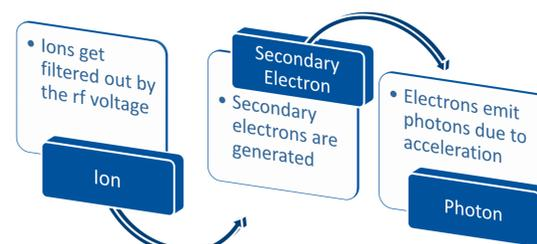
Fig. 6: Bremsstrahlung mechanism from ions to soft X-rays in a quadrupole instrument
