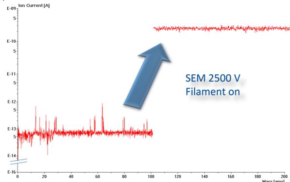
Fig. 5: The baseline goes up by 3 orders of magnitude when the filament is turned on;  $2 \cdot 10^{-2}$  mbar SPM source and  $1 \cdot 10^{-5}$  mbar analyzer pressure
