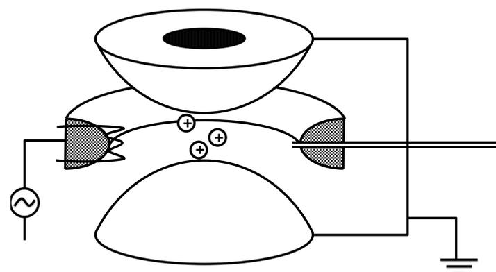
Fig. 1: Schematic of the used FT-QIT
