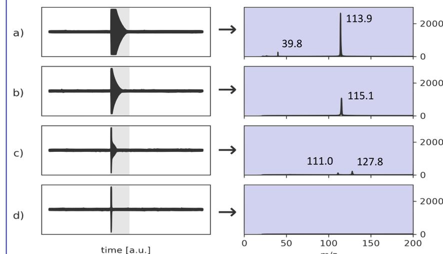
Fig. 3: Four mass spectra acquired subsequently within approx. 20 min. The plots show a decreasing signal intensity.
