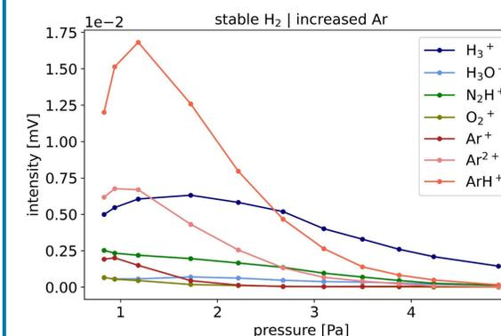
When increasing the argon pressure, the signal intensities for  $\text{Ar}^+$ ,  $\text{Ar}^{2+}$ , and  $\text{ArH}^+$  reach a maximum at 1.2 Pa. The signals of  $\text{H}_3^+$  and  $\text{H}_3\text{O}^+$  peak at 1.8 Pa. Towards higher pressures the signal intensities of all the species drop.
