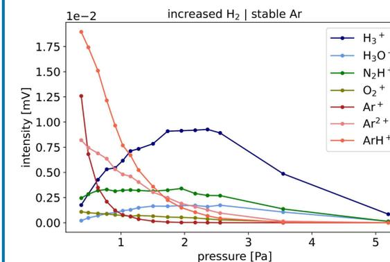
When the hydrogen pressure is increased, the signal intensities of  $\text{H}_3^+$  and  $\text{H}_3\text{O}^+$  peak at 2 Pa and drop afterward. The peak intensities of all the other species only display a decrease as the pressure rises.
