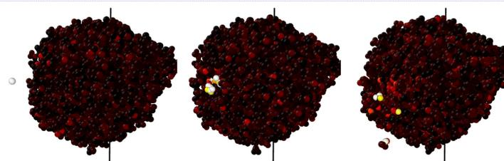
Fig. 4: Single collision with droplet. Colors depict kinetic energy of particles
