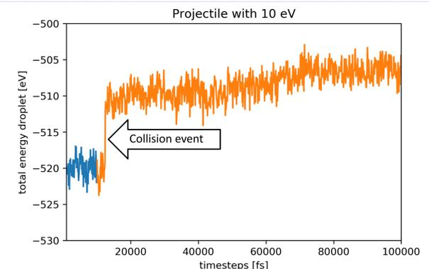
Fig. 3: Simple collision of charged droplet and an argon projectile
