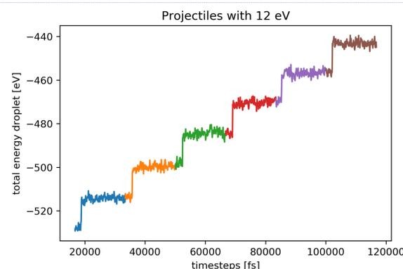
Fig. 6: Heating curves of the droplet with successive collisions
