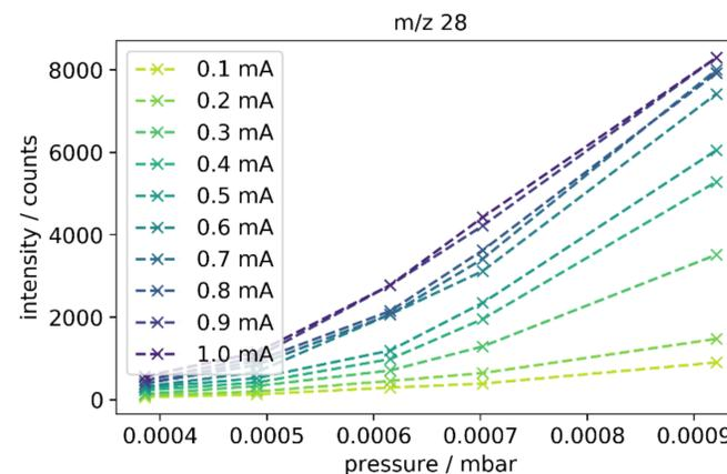
Fig. 3: Nitrogen signal goes up at higher pressures even though it should be cut off.
