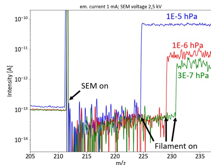
Fig. 5: The observed shift of the baseline at different pressure levels of air in the quadrupole region.
