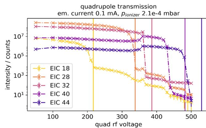
Fig. 2: At higher pressures, ions are not filtered out entirely.
