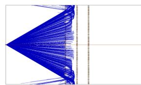
Fig. 4: Ion trajectories simulated with Simion for the close state of the Tristate Ion Shutter
