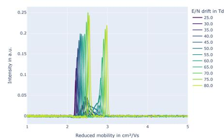
Fig. 6: variation of the reduced electric field in the drift tube
