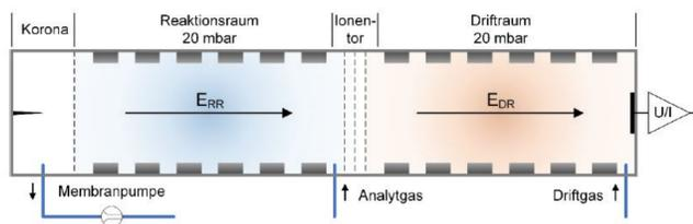
Fig. 1: Schematic overview of the HiKE-IMS. Length of reaction and drift tube is 100,5 mm and 304,5 mm[2]
