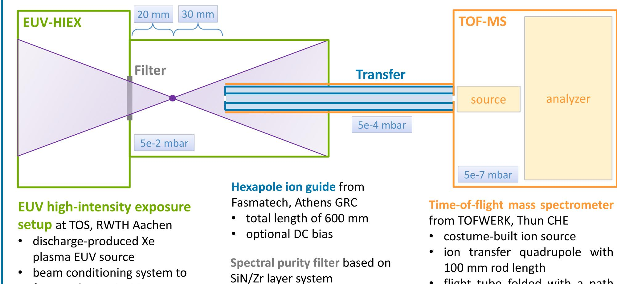
flight tube folded with a path
