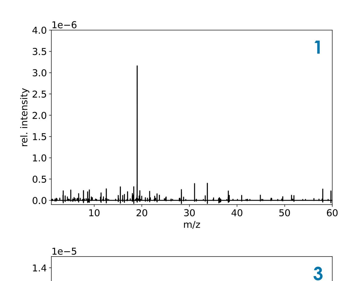
**1 - Native ions from EUV plasma** Ion signal at 3 Pa hydrogen and added DC bias in the hexapole. No  $H_3^+$  signal due to low mass discrimination, only single  $H_3O^+$  ions are detectable. Filter in use, high spectral purity.
