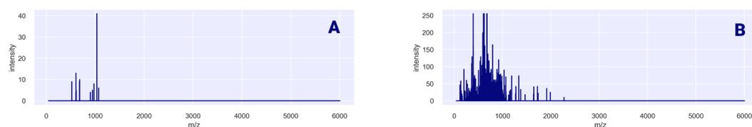
**Fig. 7** Non-summed mass spectra from the same measurement. (A) Regular spectrum with a low total sum of registered ions (550). (B) Example spectrum with a total ion count magnitudes over the regular spectrums case (~13000) which are comparably rare.
