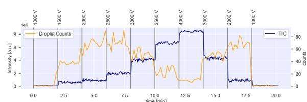
**Fig. 6** Observed dependences between droplet signature count, TIC and the variation of the capillary voltage. Other parameters suggest also a dependence of observed droplets. All parameters which are crucial for the spray generation show the highest impact on the droplet count.
