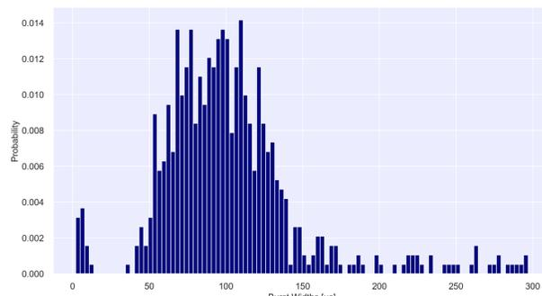
**Fig. 4** The histogram of all recorded burst widths during a long-time measurement show a distinct width distribution. We conclude that the burst widths probably depend on the location of the fragmentation of the initial compact droplet. If this fragmentation appears further down the ion stream, the burst signal becomes narrower. An earlier fragmentation and thus longer spreading occurs in a wider signal.
