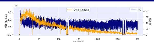
**Fig. 5** Long-term measurement of an electrospray with focus on the droplet signature count and the TIC, recorded at the microTOF MCP detector. The zero-signal at approx. 5500 seconds is reasoned by a syringe switch. The droplet count is decreasing over the time.
