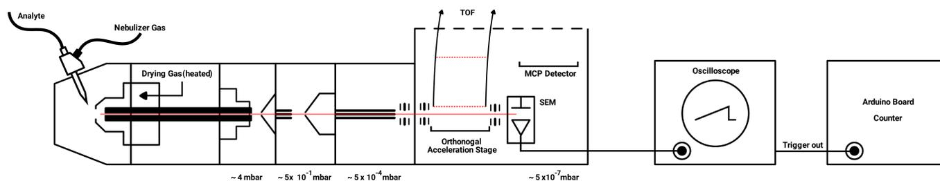
**Fig. 1** Schematic representation of the experimental setup with a Bruker microTOF and droplet signature detection
