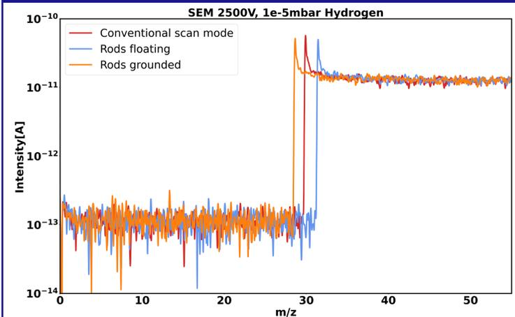
Figure 2: Baseline recorded with several operating modes of the quadrupole
