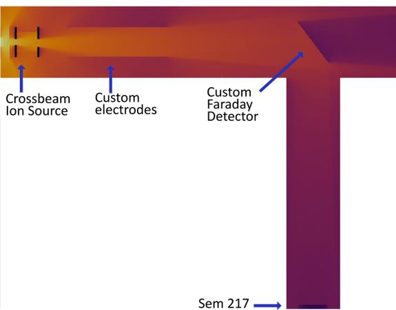
Figure 4: SPARTA simulation of particle density of metastable atoms in the mock-up system
