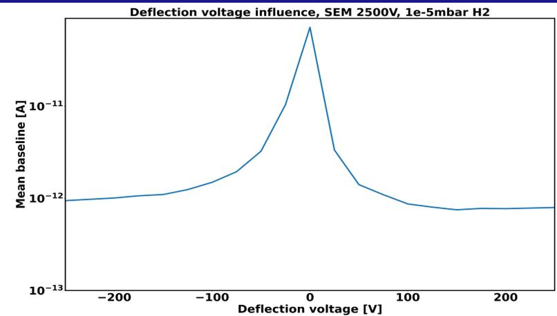
Figure 3: Influence of potentials applied downstream of the rod system on the baseline
