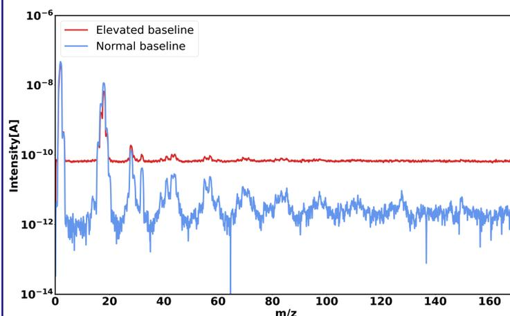
Figure 1: A normal spectrum compared to a spectrum with an elevated baseline
