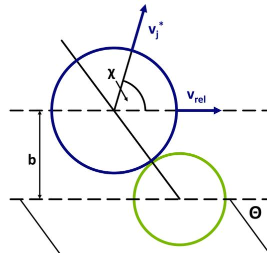
Fig. 1: Geometry of the Monte Carlo Collisions.
