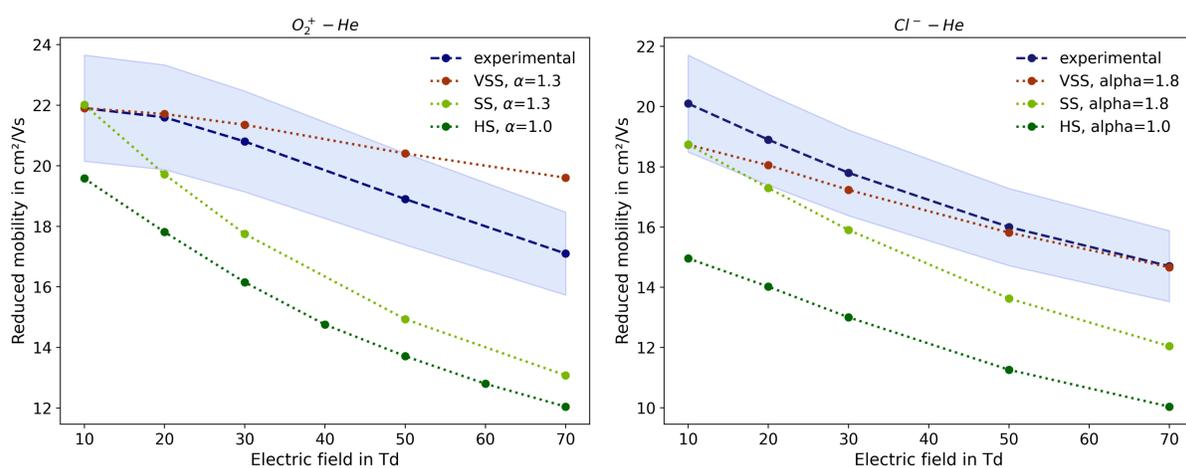
Fig. 3: Comparison of the Ion Mobilities of the HS and VSS Model with experimental results for a)  $O_2^+$  in a Helium-Matrix and b)  $Cl^-$  in a Helium Matrix.
