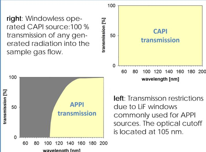
right: Windowless operated CAPI source: 100 % transmission of any generated radiation into the sample gas flow.
