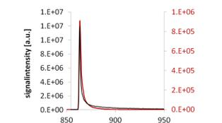
Figure 5) The tailing (analyte: caffeine) does not noticeably change for different source temperatures (red trace 50 °C, black trace 150 °C).
