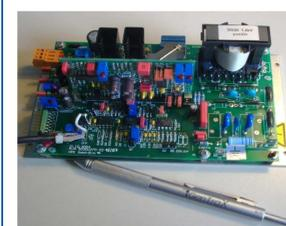
Figure 2: HV power supply
