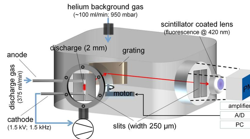
Figure 3: VUV spectrometric setup
