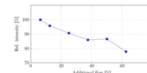
**Figure 5** The total ion count measured with an additional gas flow added concentrically to the flow of the DBD (1 slm) feeding the 5 mbar ion funnel.
