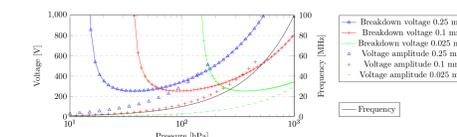
**Figure 7** The results of the 100 mbar ion funnel scaled to a broad pressure range using equations 1 and 2. Additionally the breakdown voltages for each plotted electrode distance is given.
