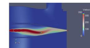
**Figure 6** A cut through the simulated flow field of the 5 mbar ion funnel with the velocity in x-direction in m/s.
