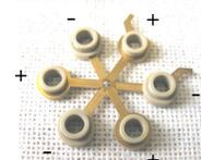
**Figure 3** The two smallest electrodes of the ion funnel with the PEEK spacers.
