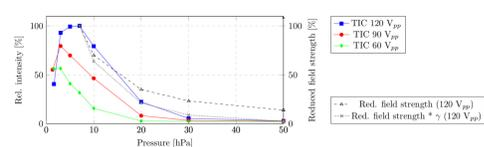
**Figure 1** The total ion count measured at different pressures and voltage amplitudes (at 1.8 MHz) applied to a funnel with an electrode distance of 0.5 mm (Stage 2, Fig 2). The second vertical axis shows the reduced field strength.
