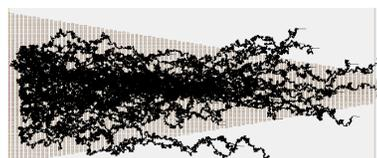
**Figure 8** A cut through the Simion SDS ion trajectory simulations of the ion funnel at 100 hPa driven with 200 Vpp and 10 MHz. In black the ion trajectories of 40 ions with mass 100 are shown.
