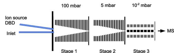
**Figure 2** A schematic drawing of the CIMS transfer stage.
