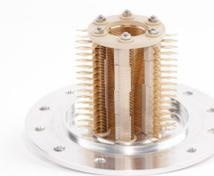
**Figure 4** A photo of the 100 mbar ion funnel before the printed circuit boards are attached.
