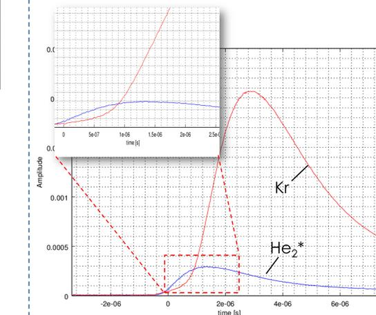
Faster formation of the  $\text{He}_2^*$  than electronical excitation of Kr. The slopes follow a characteristic pattern of a consecutive reaction, indicating fast quenching of the helium excimer by krypton.
