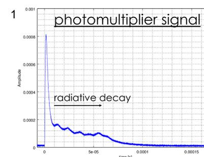
1) Time and wavelength resolved photomultiplier signal. The temporal profile follows the temporal current and voltage profile (2 and 3).
